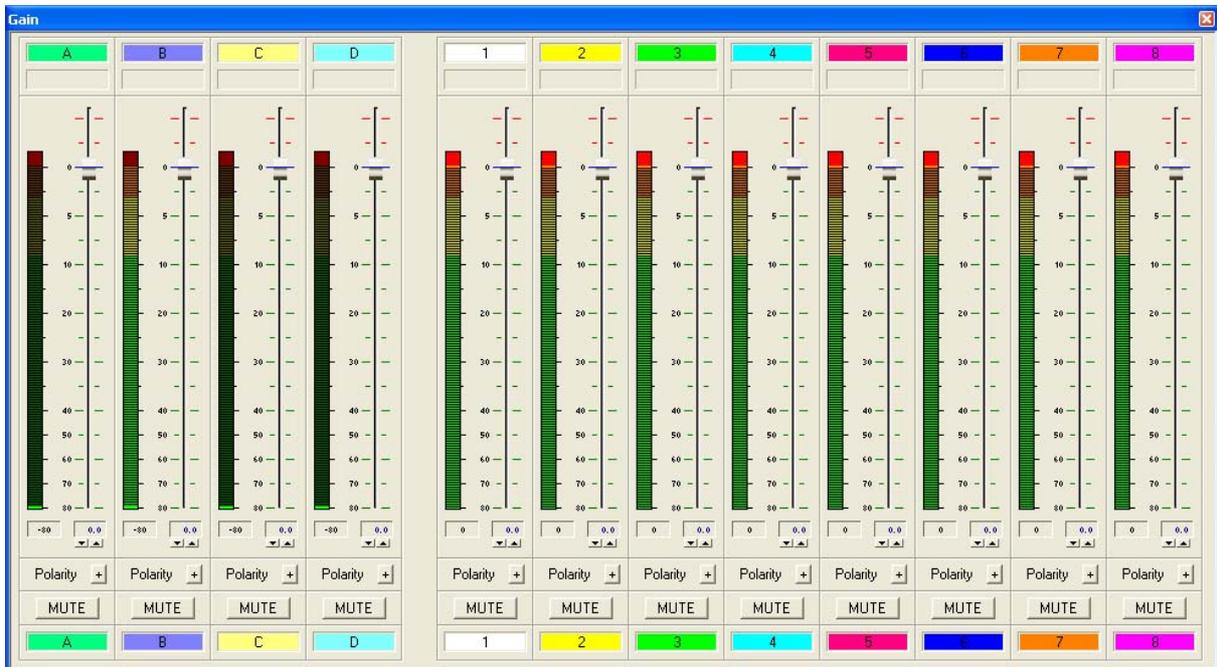
All gain buttons will open this gain overview window. Most of the functions are self-explanatory. Adjust the relevant gain by grabbing the fader and moving it, by using the up/down arrows or by entering the correct value with the keyboard.
