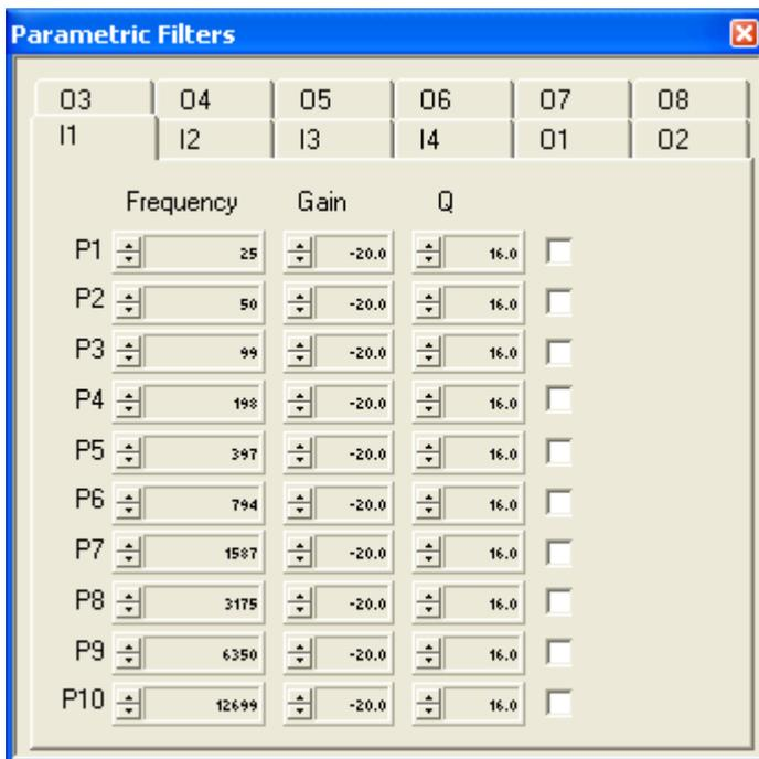
10 full parametric filters are available on every input. 8 full parametric filters are available on every output. All the [Par] buttons (on in and outputs) will open this same window. You can select the relevant input or output by selecting the corresponding tab. You activate a parametric filter by selecting it on the right hand side. When you select a filter, a graphic representation will appear in the graphic window of the relevant input (output). You can now
