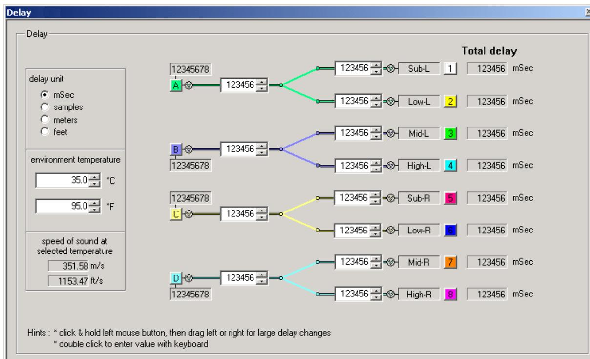
All the different [DELAY] buttons will open this same window which gives you an overview of all your input and output delay settings. You can set the delay for each input and output in different ways:
