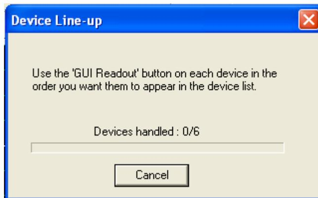
Now press on the [GUI Readout] button from the Intelli-Q/X that is located on the top. Do this also for the device that is located underneath the top Intelli-Q/X. And do so for all the devices you have, systematically going down to the bottom device.
