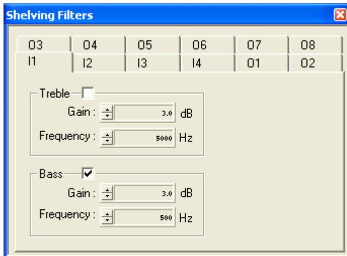
You should be now being able to figure out for yourself how it works. It is always the same logic: you can select the relevant input or output via the tabs. Hi and Low shelving are available on all inputs and outputs. Again: selecting a high or low shelving filter will make it appear in the relevant graphics screen. Grab the handle and you can adjust the curve.
