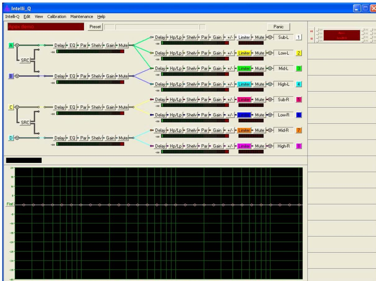
If you are used to work with the Apex Intelli-Q, you will have no problem getting used to the Intelli-X, the same logic has been applied. In the top left of the screen you see the name of the device you have selected with the mouse from the list on the right of the screen. Click in the red name field to be able to alter or change the name.
